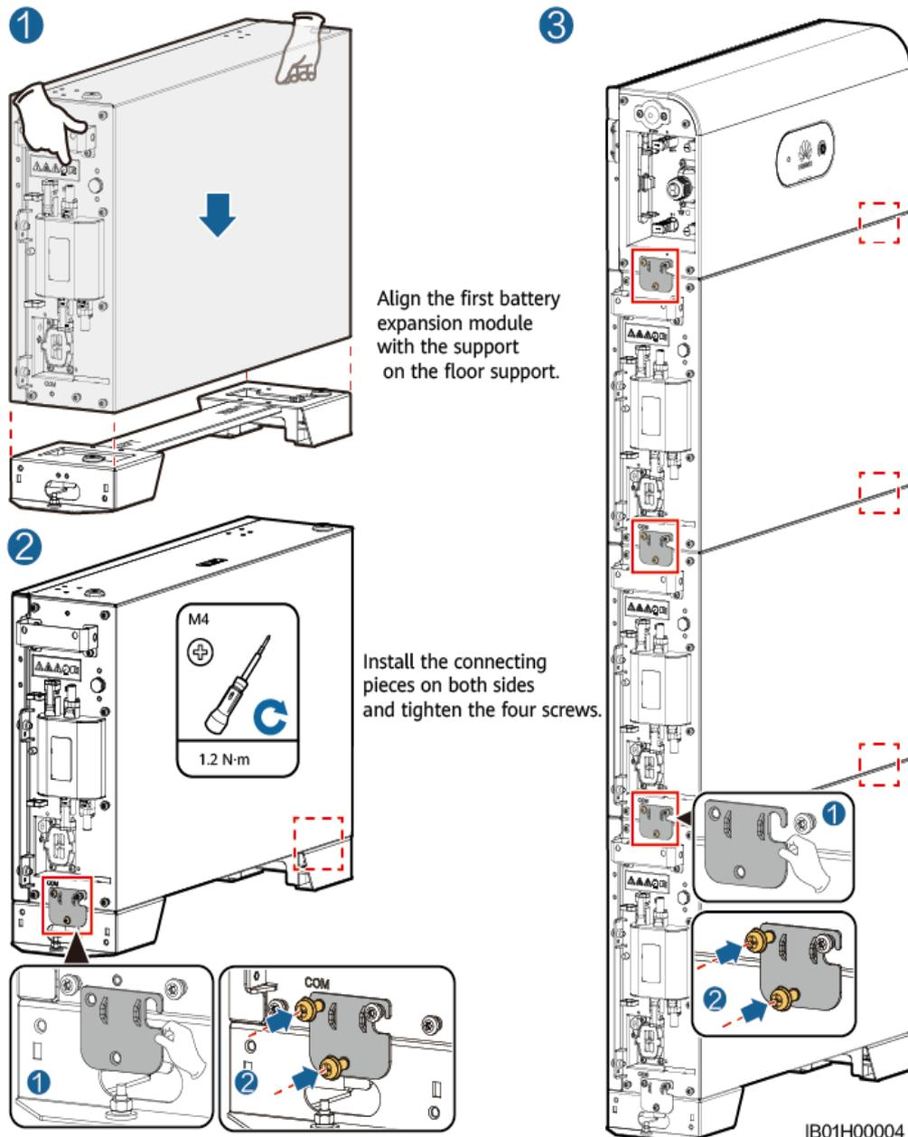
Align the first battery expansion module with the support on the floor support.
